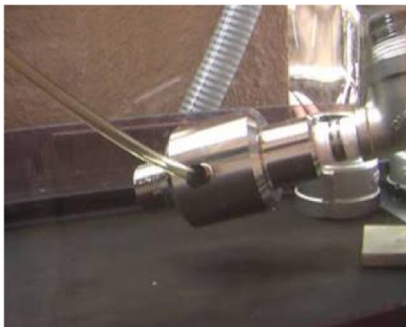
Fig. 2: Using 60L/min OK Nozzle for the silicon wafer ultra-mirror polishing
