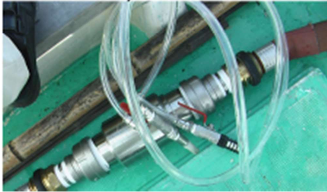
Used 500L/min OK nozzle
